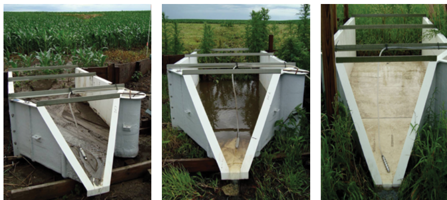
These flumes measure surface water runoff from the STRIPS watersheds. Note the amount of sediment displaced from a 100 percent no-till crop field (left) compared to a field enhanced with 10 percent prairie (center) and a field of 100 percent prairie, which has little sediment loss.
